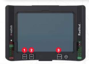
DELAY setting, return time 1 SENS setting, sensor sensitivity 2 SHADE setting
